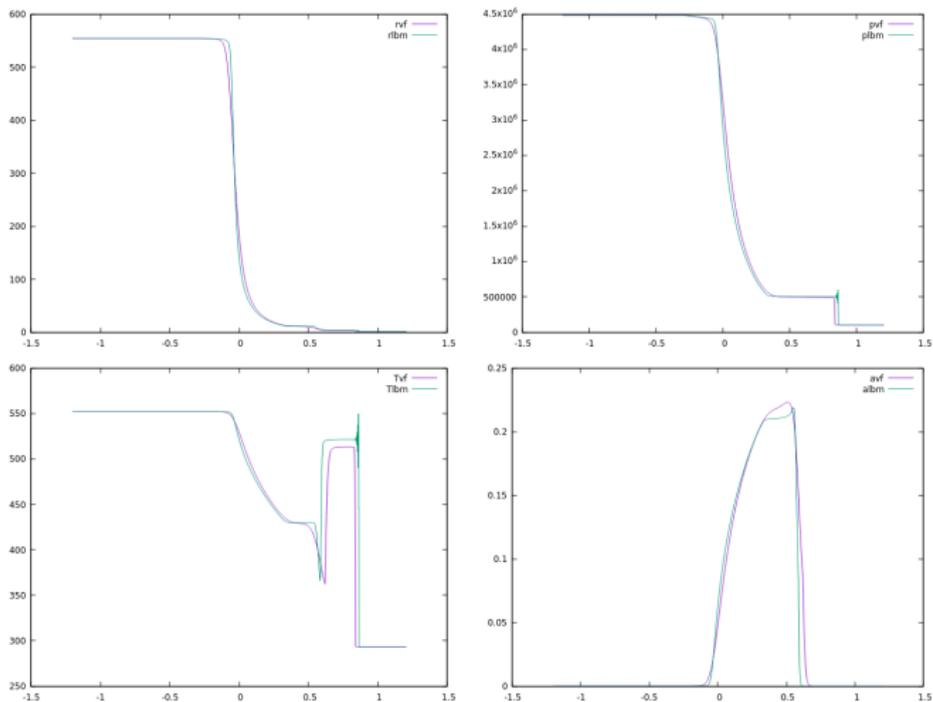
Top left: density, top right: pressure, bottom left: temperature, bottom right: vapor mass fraction. Comparison between the Finite Volume and Lattice Boltzmann Method with  $\omega = 1.9$  on a mesh with 2000 cells.
