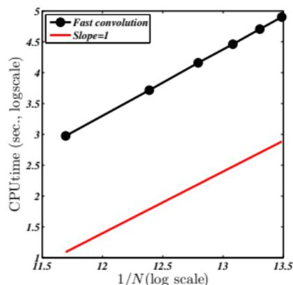
**Figure:** Computational time for the evaluation of the convolution by the fast algorithm vs  $N$  (for  $M = 160$ ). The total number of time steps  $N$  increases from  $N = 1.2 \times 10^5$  to  $N = 7.2 \times 10^5$ , with step  $1.2 \times 10^5$ . We observe a slope equal to 1, showing that the cost is linear according to  $\log(1/N)$ , i.e. as  $\mathcal{O}(N \log N)$  for the computational time.
