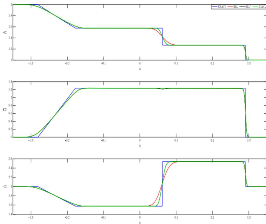
FIGURE – Dam break Problem . Plots of the variables using  $HLL$ ,  $HLL^*$  and  $HLLC_{\bar{u}}$  solvers for 1000 grid cells
