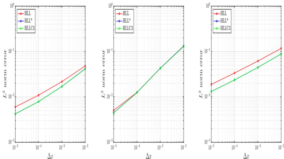
FIGURE – The Dam break problem : Convergence of  $L^2$  norm errors at  $t = 0.05s$  with mesh refinement for  $h$  on the left, for  $\bar{u}$  in the middle and for  $\hat{u}$  on the right.
