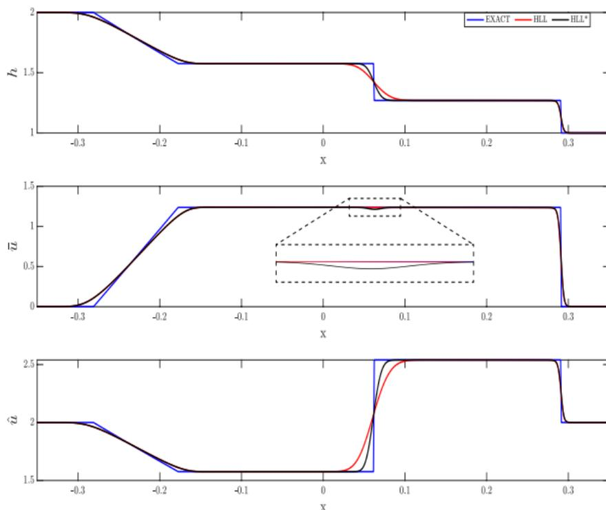
FIGURE – Dam break problem. Plots of the variables using  $HLL$  and  $HLL^*$  solvers for 1000 grid cells
