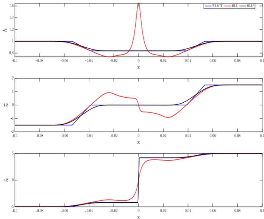
FIGURE – Two rarefactions case. Plots of the variables using  $HLL$  and  $HLL^*$  solvers for 1000 grid cells
