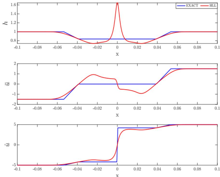
FIGURE – Two rarefactions case. Plots of the variables using *HLL* solver for 1000 grid cells
