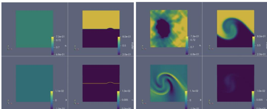
From top-left to bottom-right : Pressure, volumic fraction  $\alpha$ ,  $\omega = \frac{D_t \alpha}{\rho \gamma \Sigma^2}$ ,  $z = \frac{\Sigma^{2/3}}{\rho^{1/2}}$ .
